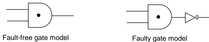
Figure 12. Faulty And gate model made of fault-free And gate and an inverter for fault insertion
